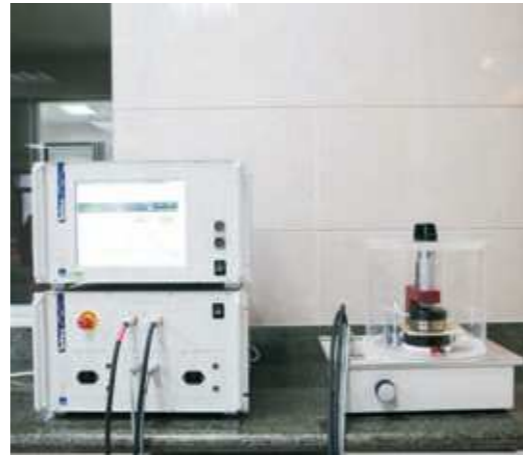
High accuracy analyzer for oil and solid insulation materials imported from Swiss
