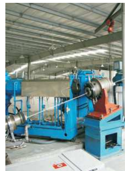
35kV Triple Extrusion Rubber CV Production Line
