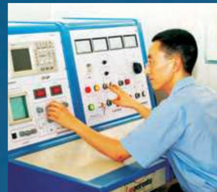
Partial Discharge Withstand Voltage Control System
