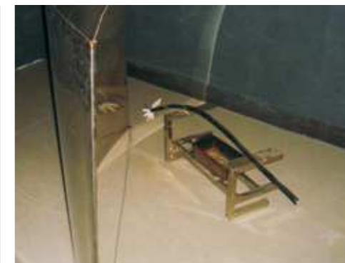
Smoke Density Test Apparatus for Completed Cable
